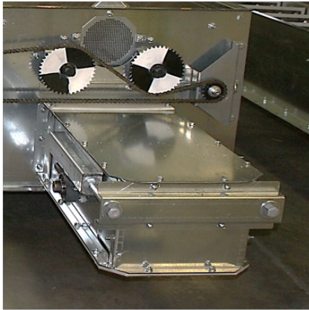
Fig 3 Tub Drag Conveyor
