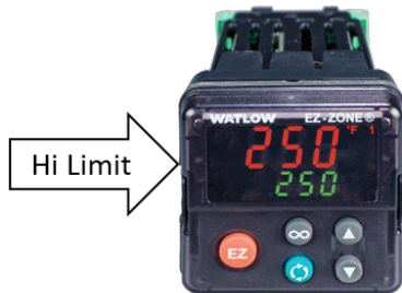
Fig 11 Hi Limit Control
